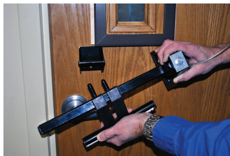
Place hooks on quick release bracket. Allows responders to unlock with security key.
